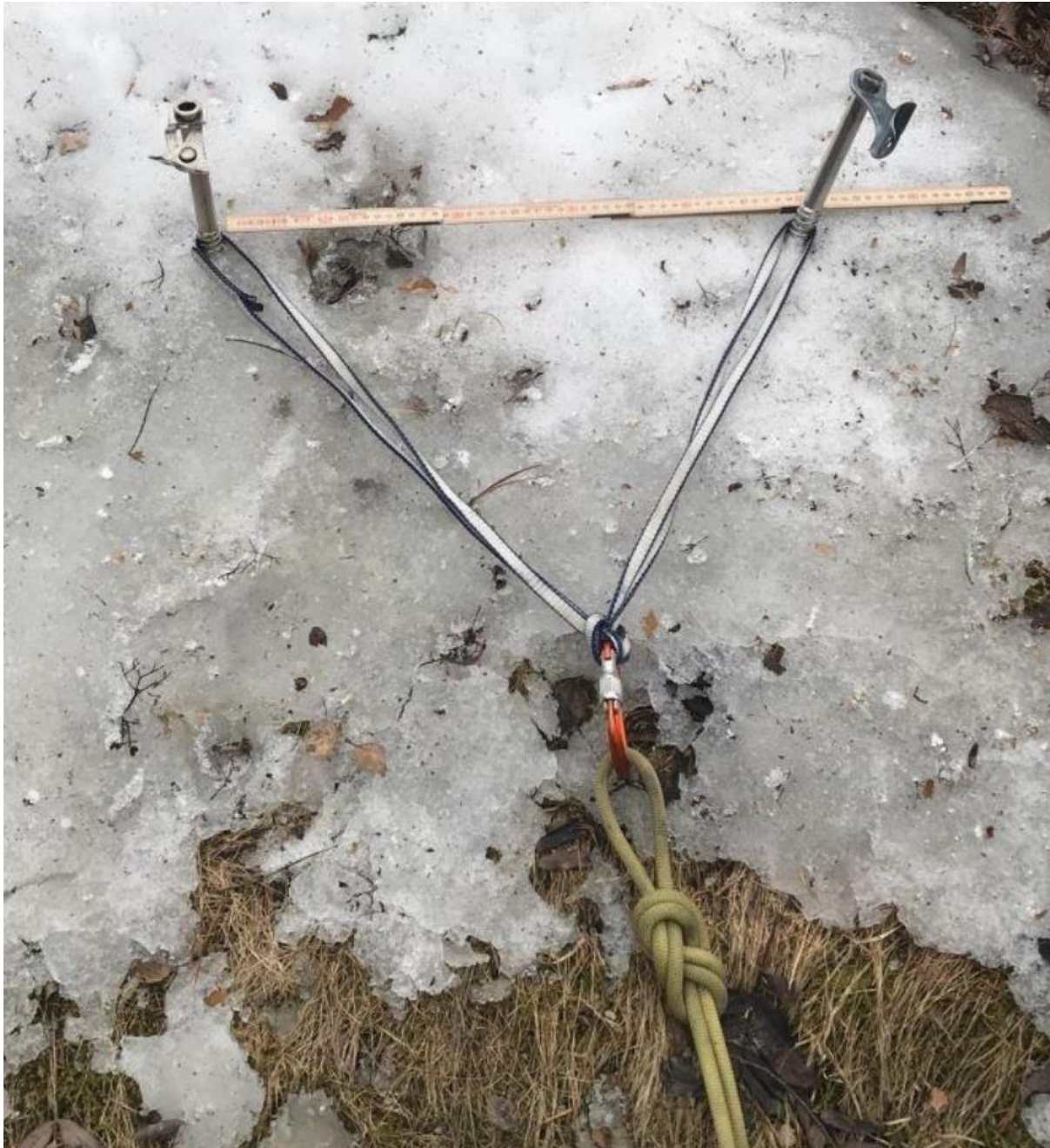
Ice screws should be screwed all the way in (here there was thin ice over the grass), and the sling should be attached by carabiner to the screws
